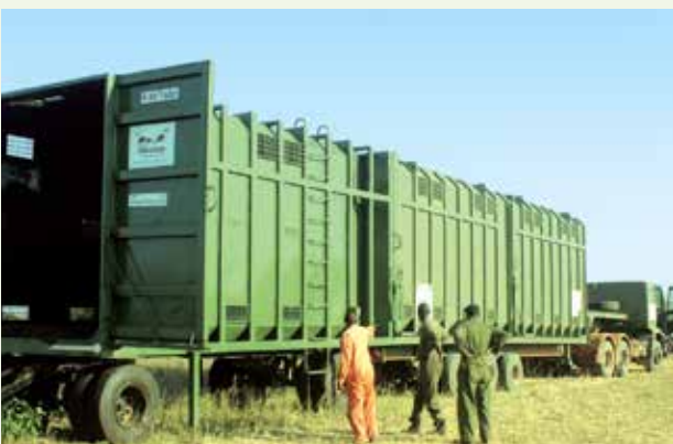
7. The translocation vehicle, called the Prime Mover, is made up of three containers. The first is used to place the captured pachyderm and stimulate it to wake up. It is then driven into the second container and the sliding door is shut to make way for the next elephant. The trumpeting inside what is effectively a huge tin can after arousal is extraordinary.
